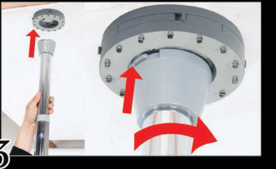
Figure 5 Raise the pole up to the ceiling mounting plate and place it in the opening of the coupling plate. Twist the pole clockwise until it locks into place in the ceiling mounting plate. You're now ready to adjust the height of the pole using the built-in spring inside of the extendable pole.
