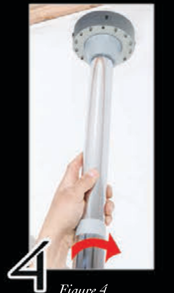
Figure 4 Twist the pole clockwise until the non-skid rubber stopper is firmly secured to the ground. With each clockwise twist of the pole, the length of the pole extends, making it tighter and more stable with each twist. When you can no longer twist the pole any longer, the pole is ready to test out. Make sure the pole is perpendicular to the ceiling and test the pole for tightness and stability before use. Once you are confident the pole is properly installed, you're ready to give it a try.
